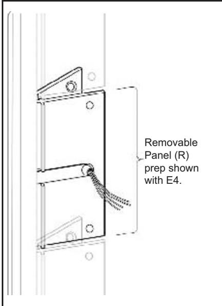
**PREPS:** PBB geared continuous hinges can be prepared with removable hinge leaf panels to allow easy access to electrical components without removing door.
