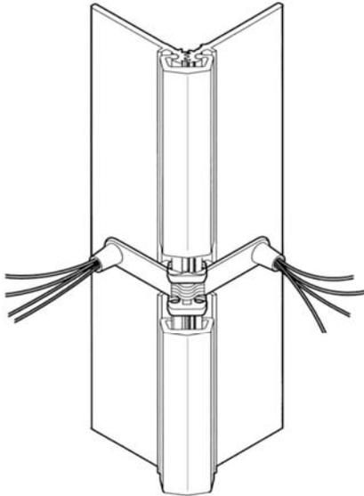
**PREPS:** PBB geared continuous hinges can be prepared for concealed electric through-wires to provide continuous current. Through-wires available in sets of 4, 5, 8 or 10 (12-wire sets available upon engineering approval). 22 gauge wire with 8" leads (approx). 120V AC/DC at 3-6 amps per conductor.
